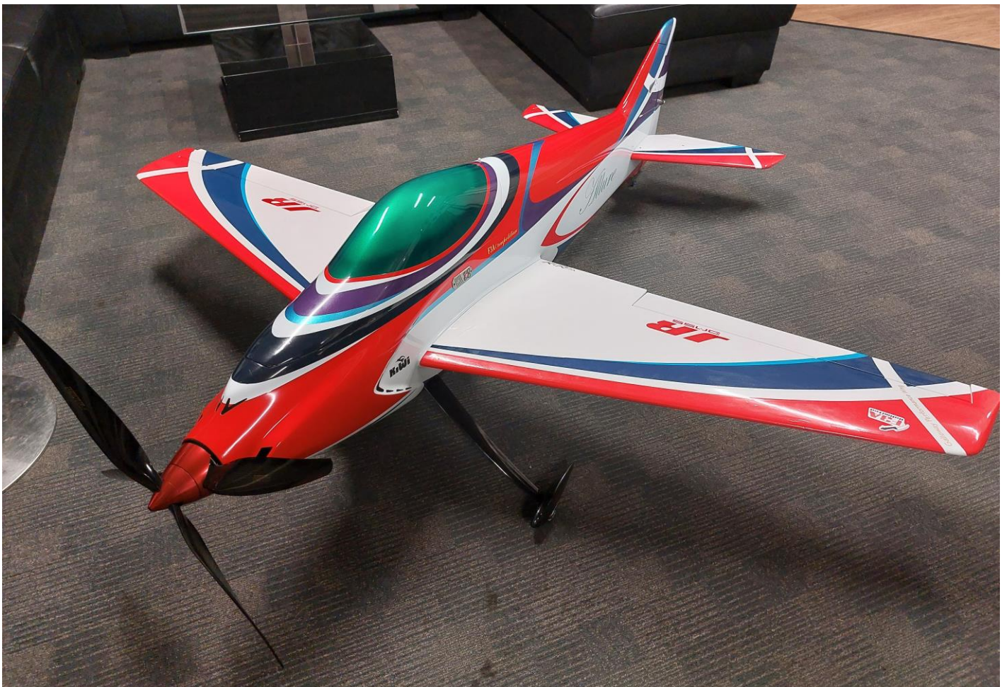
Above – Chris Eeles “Allure” ( note the counter rotating popeller which is in the spinner)
